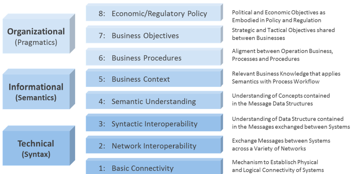
FIGURE 17 THE THREE MAIN LEVELS OF INTEROPERABILITY AND EIGHT INTEROPERABILITY CATEGORIES AS DEFINED IN [2], WITH EXAMPLES OF EACH CATEGORY
