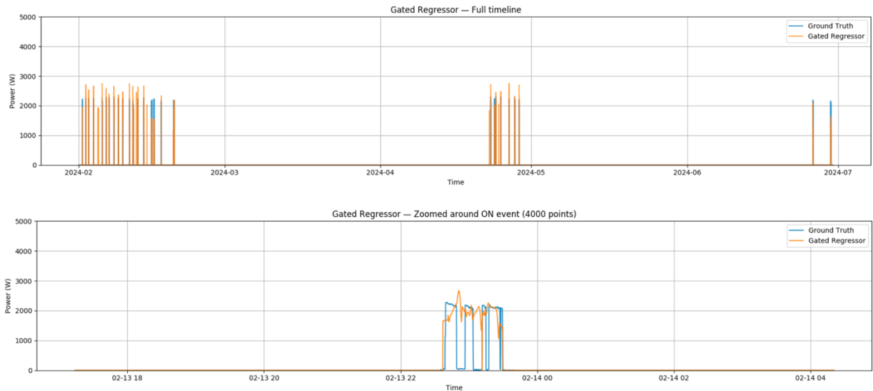
FIGURE 19: NILM PERFORMANCE USING THE GATED SEQ2POINT MODEL FOR A DISHWASHER: TOP – FULL TIMELINE COMPARISON BETWEEN GROUND TRUTH AND PREDICTED POWER CONSUMPTION, BOTTOM – ZOOMED-IN VIEW AROUND AN ACTIVATION EVENT.
